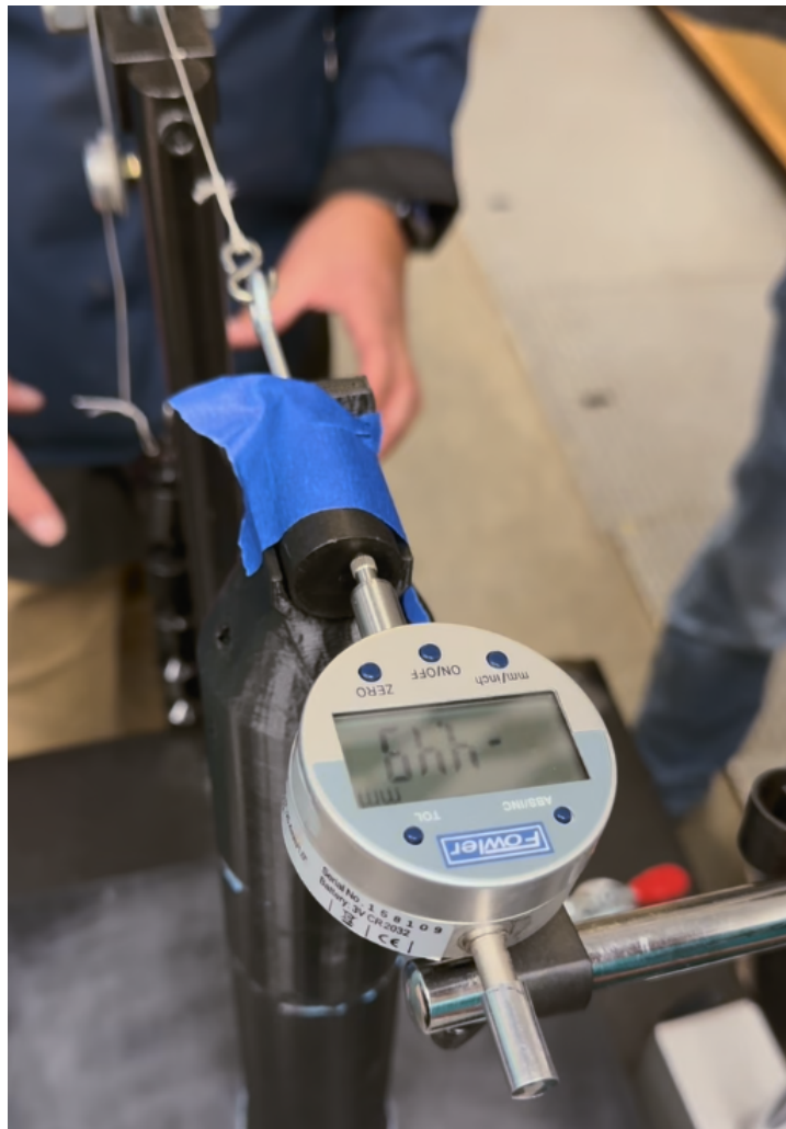
Figure 31: Picture of Displacement Sensor During Displacement Testing
