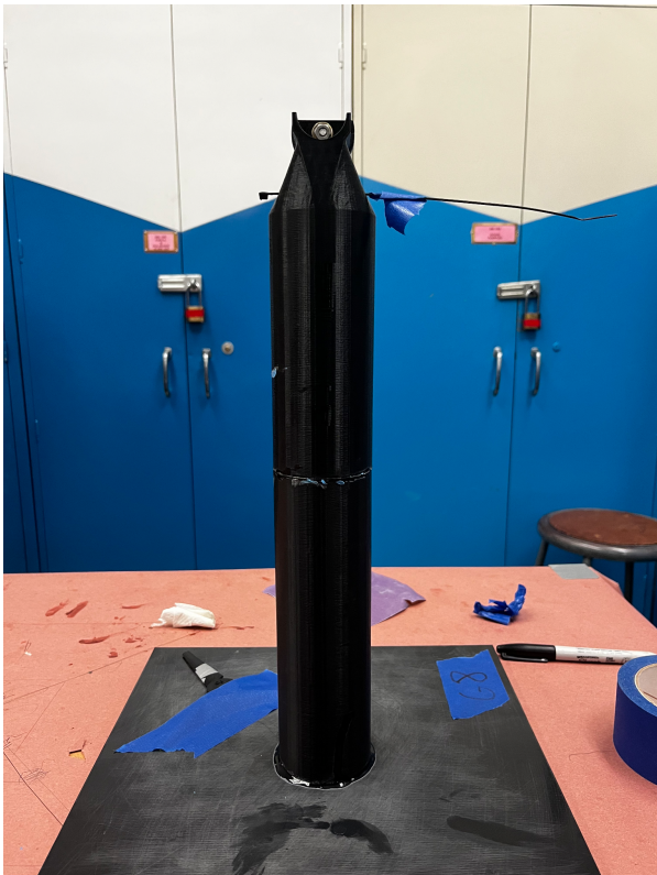
Figure 1: Final 3D printed tower after gluing.
